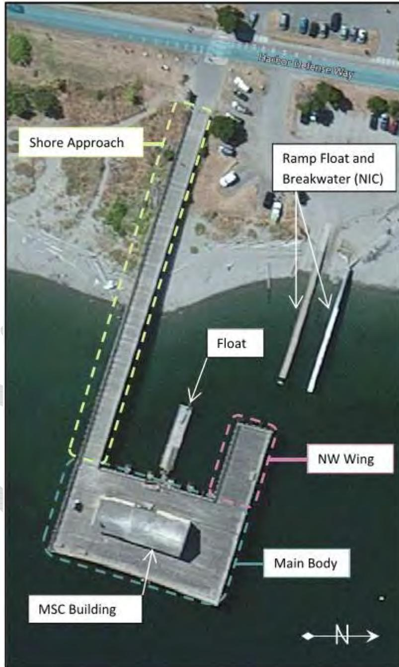
Figure 1 Existing Pier Layout and Naming Conventions
