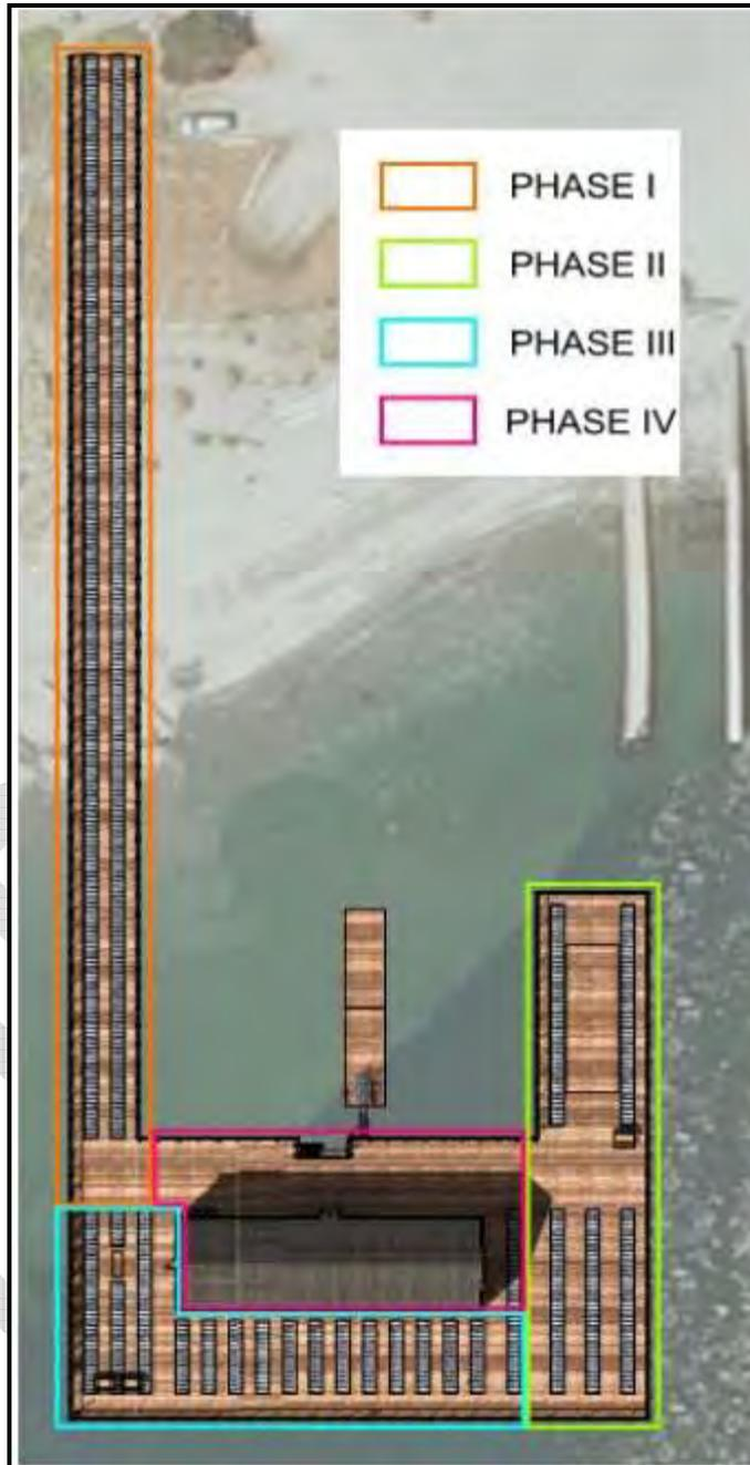
Figure 11 Schematic Pier Construction Phasing Plan
