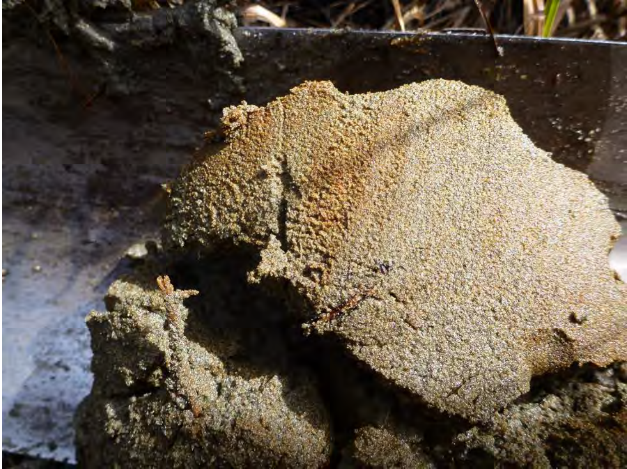
Figure 13. Close-up photo of redox concentrations at SP-A17
