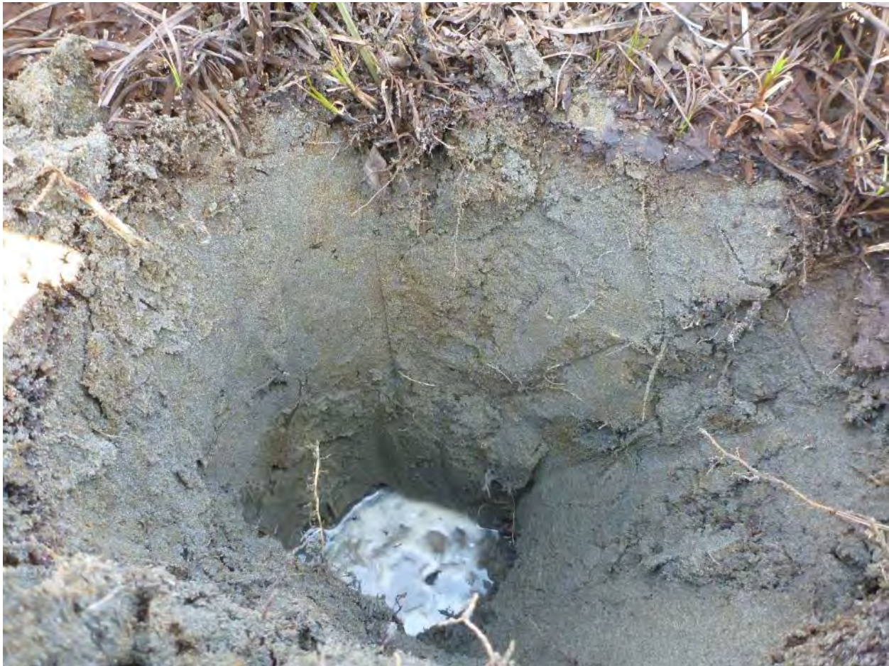
Figure 12. Photo of hydric soil indicator S5 (Sandy Redox) at SP-B1
